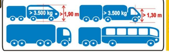
Motor vehicles with four or more axles (including the trailers' axles), with height over 1,3 m measured at the first axle, with maximum allowed mass over 3.500 kg.
